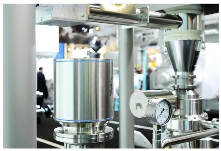
Bühler drives the pumps, dosing units and a centrifugal stirrer on their JetMix Preferment Machine with AKMH™ Stainless Steel Servo Motors from Kollmorgen
